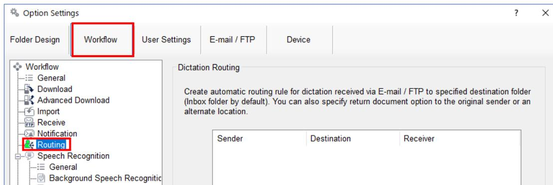
In the 'Dictation Routing' section, press the [Add...] Button to create a routing rule.
